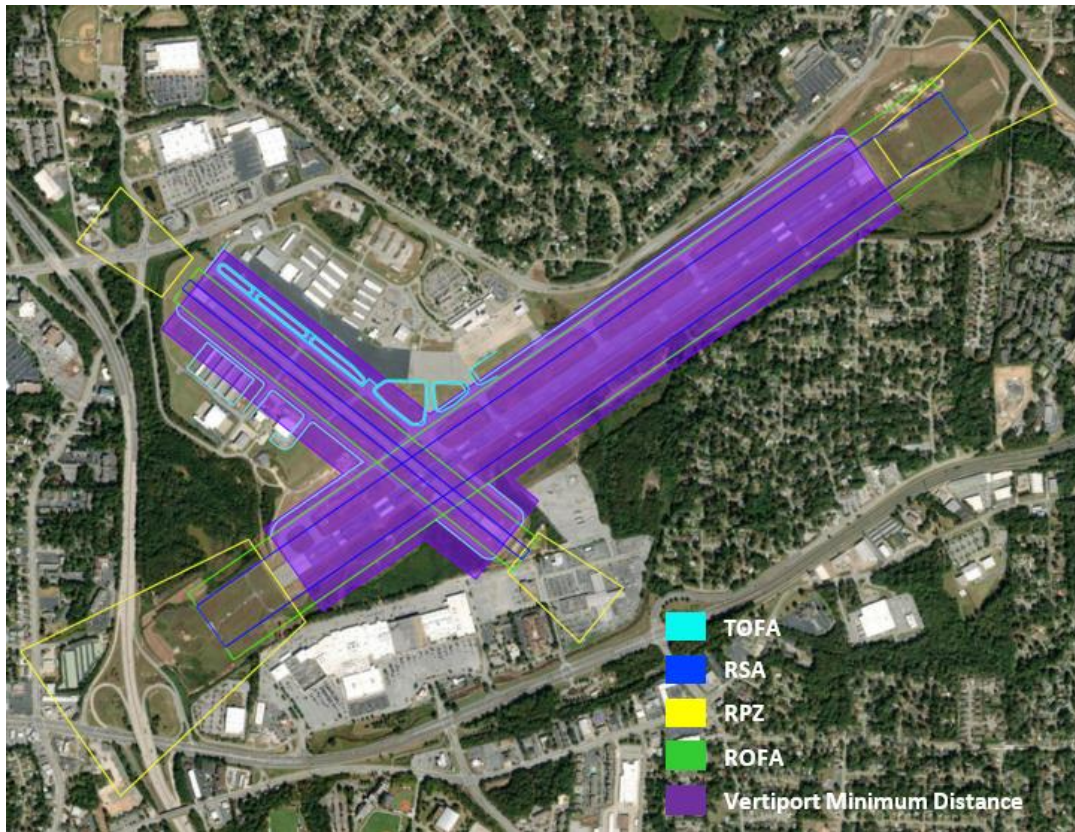
Figure 2-7: CSG Critical Airport Design Components
